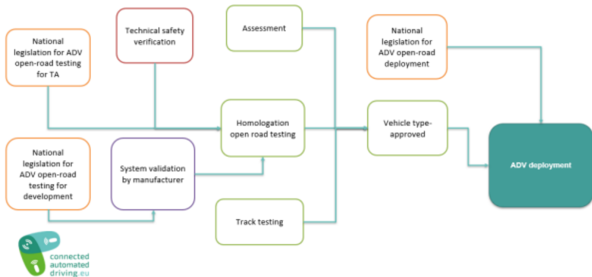
Figure 1: Framework for development, certification and deployment of Automated Driving Vehicles (FAME project)
