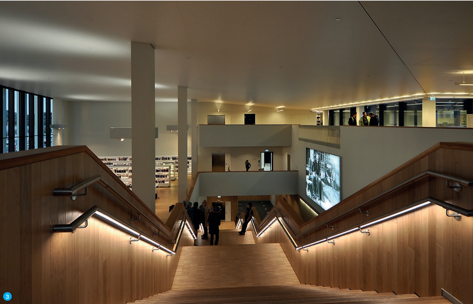
LIGHT IN THE DARK: 1) Entrance to the cultural centre in Bodø, with integrated LED lights in the stairs. 2) Handrails with integrated light, as shown in this stairway, make it easier to orientate oneself both in the library and the concert hall. 3) The light intensity is adapted to the different areas. The corridors have 200 lux, and the use of hot and cold light tones vary throughout the day. 4) The bookshelves in the library have extra strong light, and reading lights can be adjusted up to 800 lux. (Photos: Bjørnar Tønne/Byggenytt)
