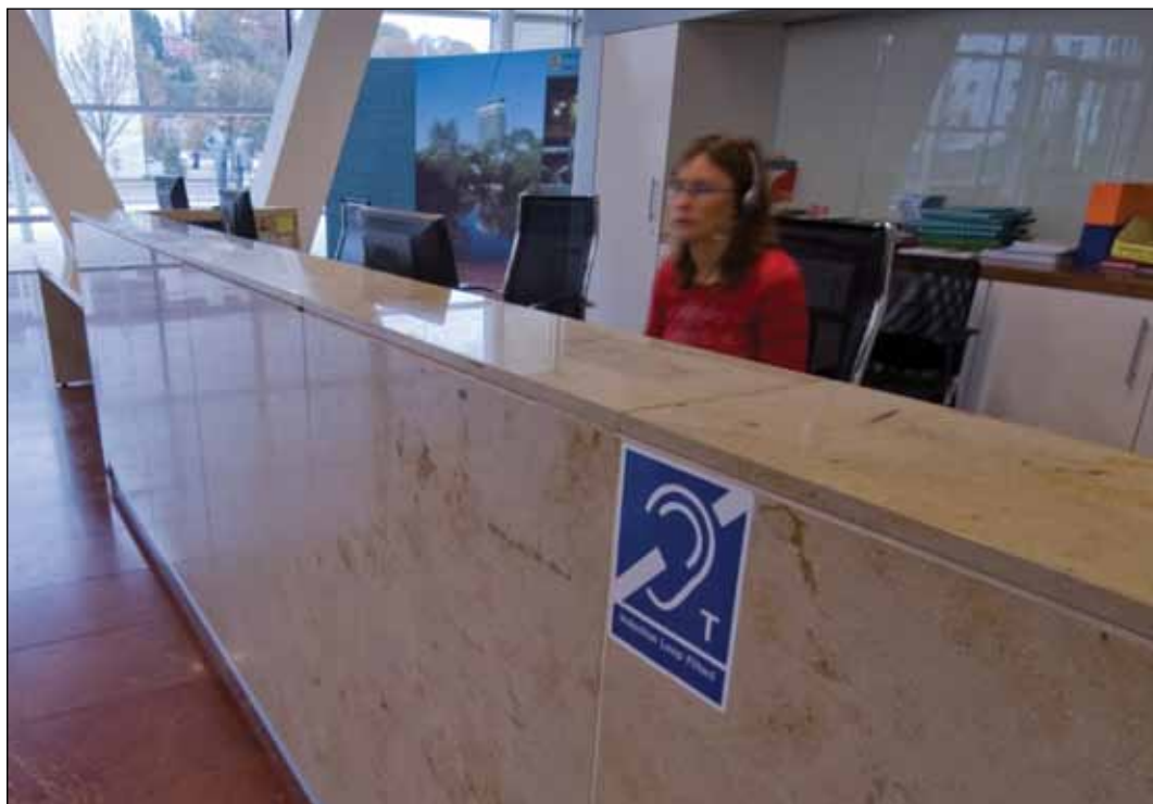
Image 4.12 Example of induction loop sign at a reception desk.
