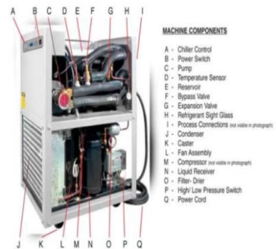
Packaged refrigeration chiller
