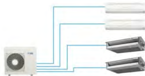
Figuur 7-4: Principe multi-split systeem, Bron: Green-r
