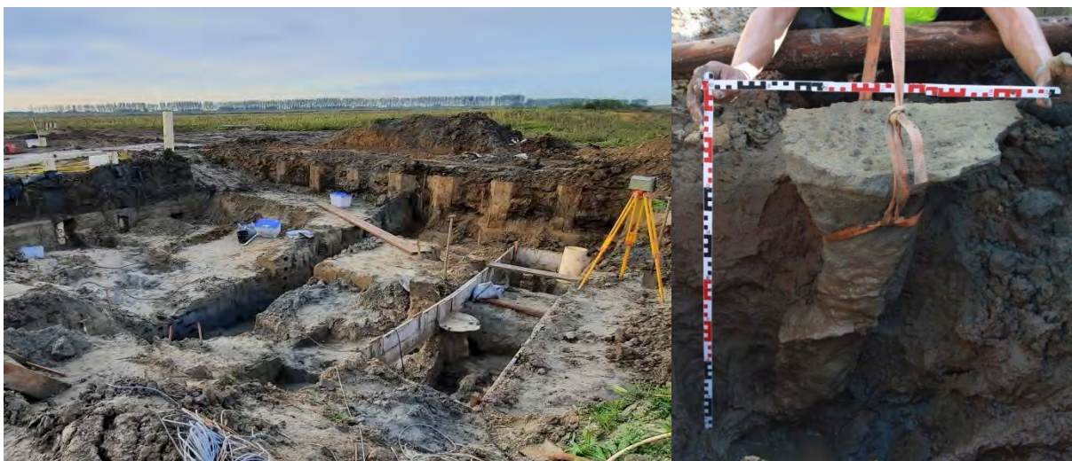
Figure 7: Left: Overview of the excavated northern test site during excavation phase of the experiment. Right: The hardened exit hole in the field.
