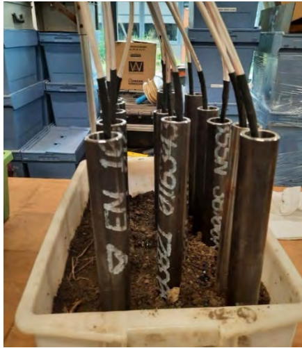
Figure 6: CPT cones with the attached DTS-cables. The cables were spliced together in order to make a loop. The heating cables were also looped.
