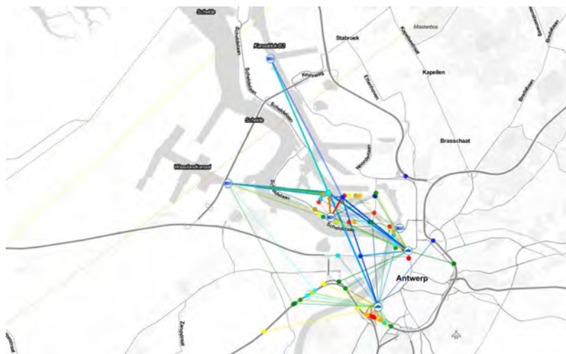
Figure 4: Example of a trip in Antwerp with an FTD, marked are the connection lines to each available gateway
