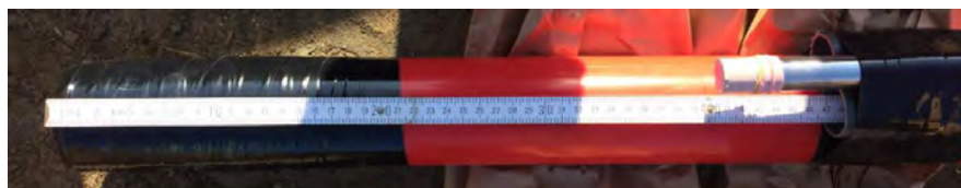
Figure 6: Fully grouted pore water pressure sensors attached to the inclinometer casings
