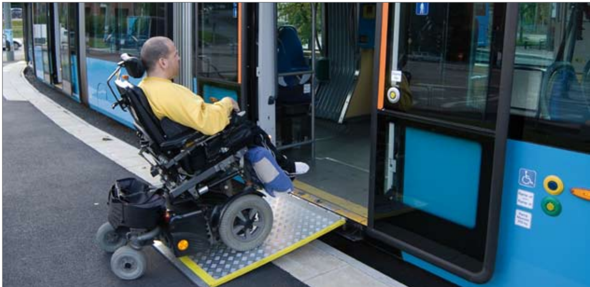
New electric ramps makes it easier to travel with heavier wheelchairs.
