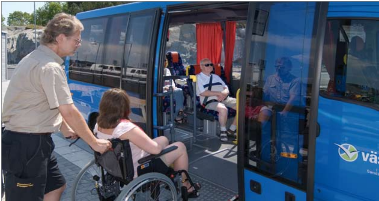
Flexline mini buses have low floor and a ramp.
